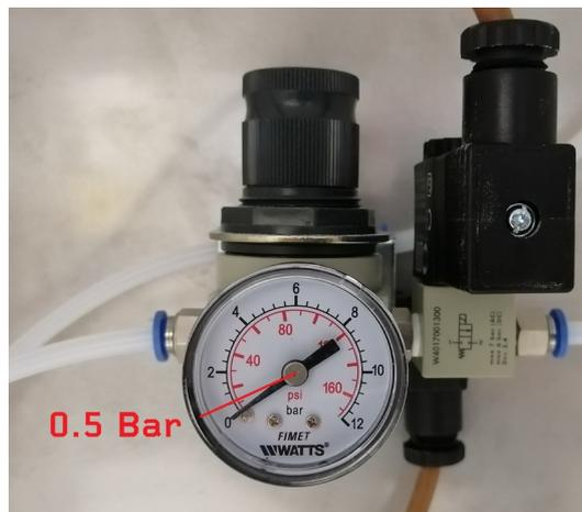
The IN gas solenoid valve, injects the gas into the lower part of the chamber, under the pistons and is equipped with a gas heater that could be used for experimental processes. The OUT gas solenoid valve extracts the gas on the upper part of the chamber, it is usually open only when the machine makes the first injection.
