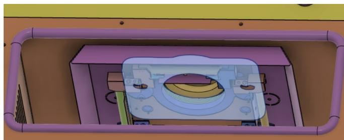
The plate is in direct contact with the internal environment of the chamber and does not suffer long thermal exposure to the chamber temperature.
