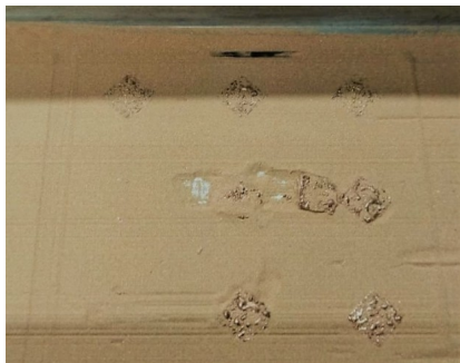
Fig. 2 A failed print, the fused material did not attach to the plate and moved around.
